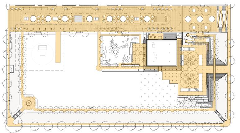
Figure 15: 2020 site plan showing impervious surfaces in orange
