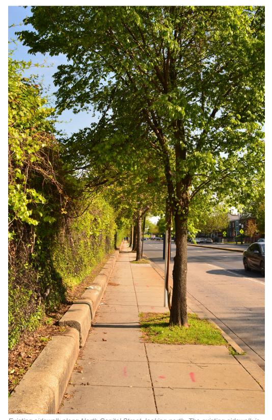
Existing sidewalk along North Capitol Street, looking north. The existing sidewalk is less than 7 feet wide, pinching to less than 3 feet at tree pits.
