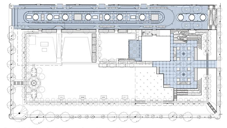
Figure 16: Updated site plan showing areas of permeable pavers in blue.
