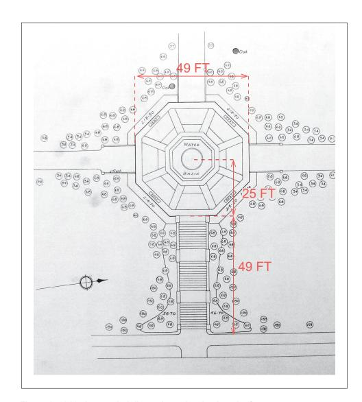
Figure 6: 1911 plan, scaled dimensions showing length of run at stone steps, distance from top landing to center of fountain plaza, and width of plaza (NTS)
