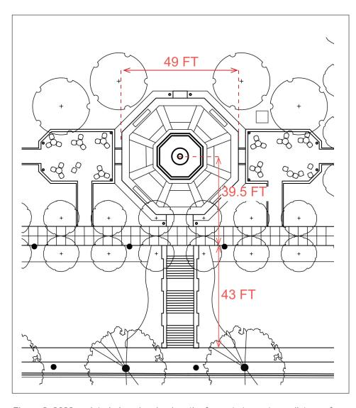
Figure 8: 2023 updated plan showing length of run at stone steps, distance from top landing to center of fountain plaza, and width of plaza (NTS)
