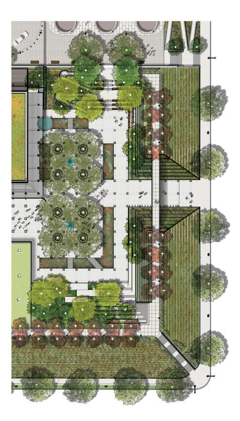
Figure 10: Plaza layout showing configuration of bioretention basins, as shown to the CFA. June 2020
