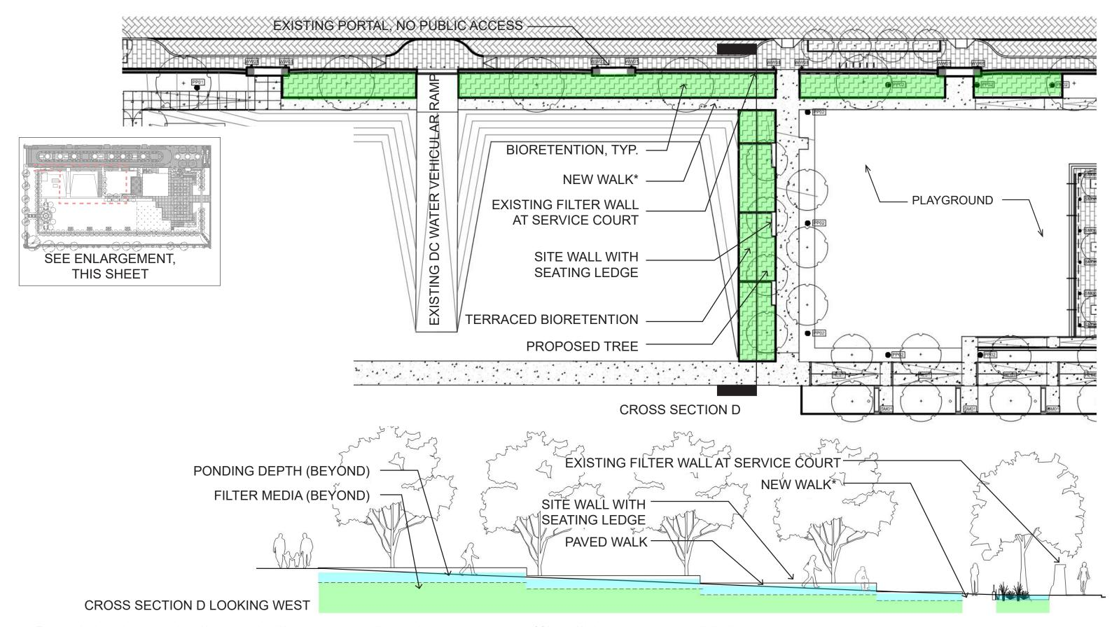
Figure 14: Updated site plan showing added bioretention. \*Note new east-west walk connecting playground to west leg of Olmsted Walk and western portal, paralleling the new bioretention basin.
