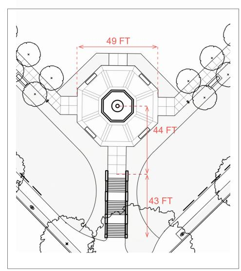
Figure 7: 2020 approved plan showing length of run at stone steps, distance from top landing to center of fountain plaza, and width of plaza (NTS)
