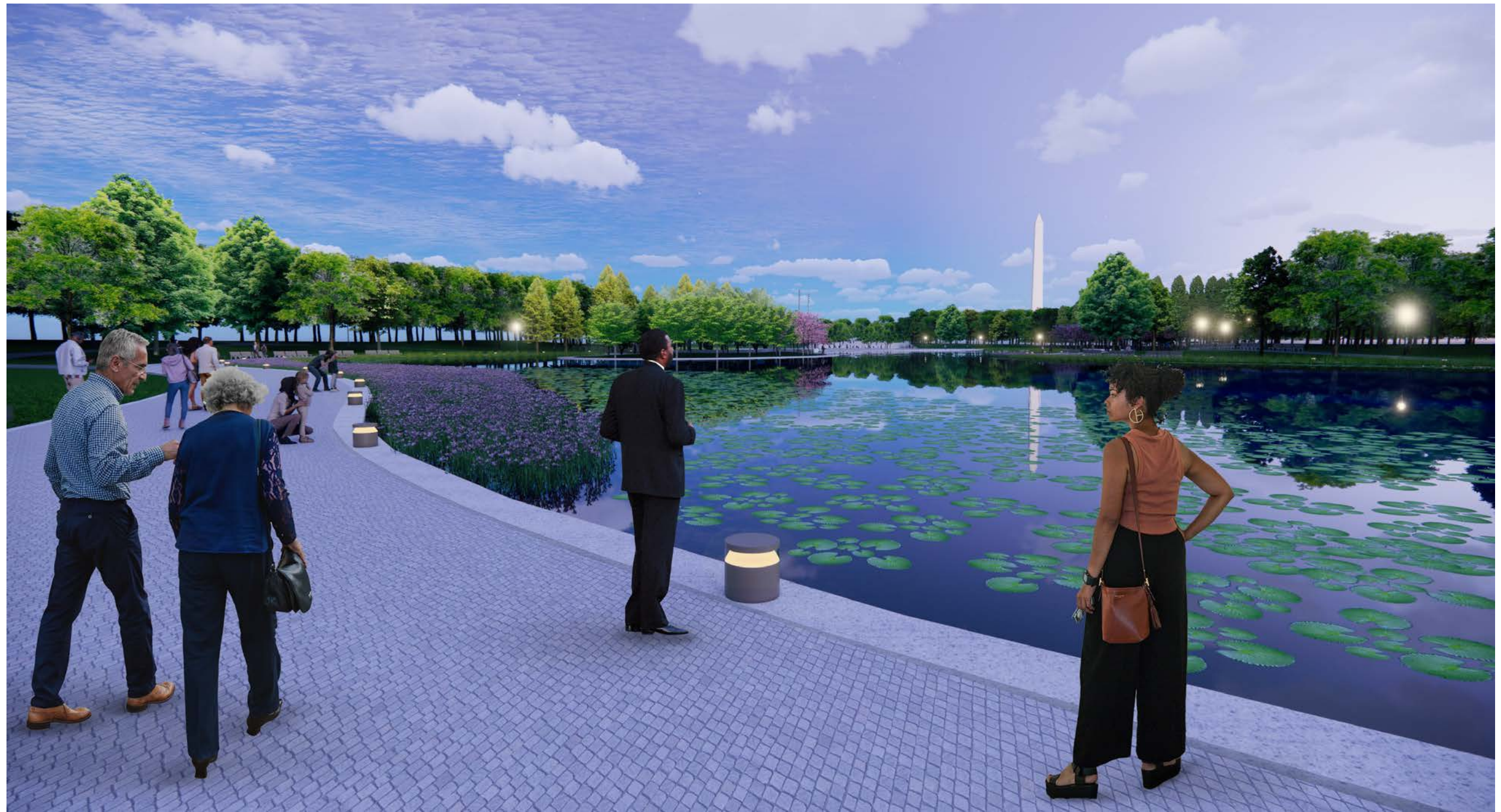
LOW PROFILE LIGHTING ELEMENT SET IN LAKE EDGE STONE, APPROX. 14" TALL, 14" DIAMETER
