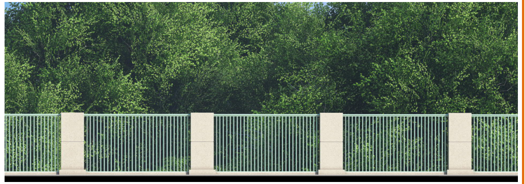
Concrete Post with Metal Handrail - Elevation
