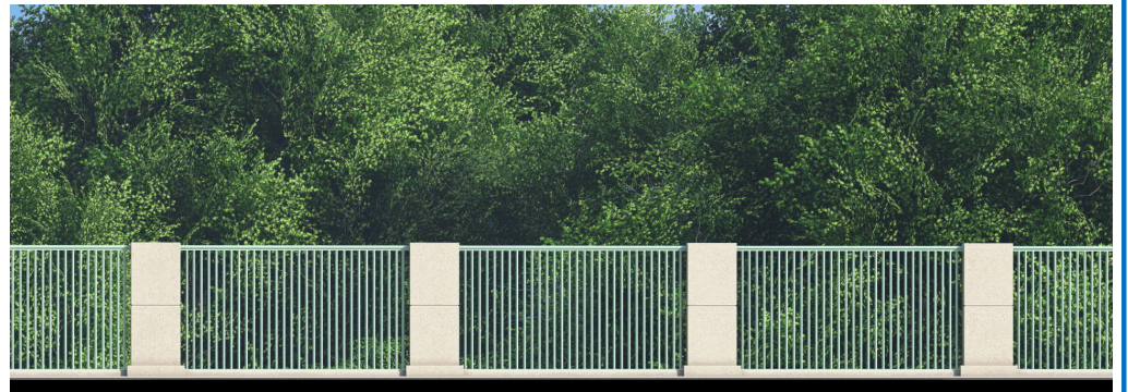
Concrete Post with Metal Handrail - Elevation
