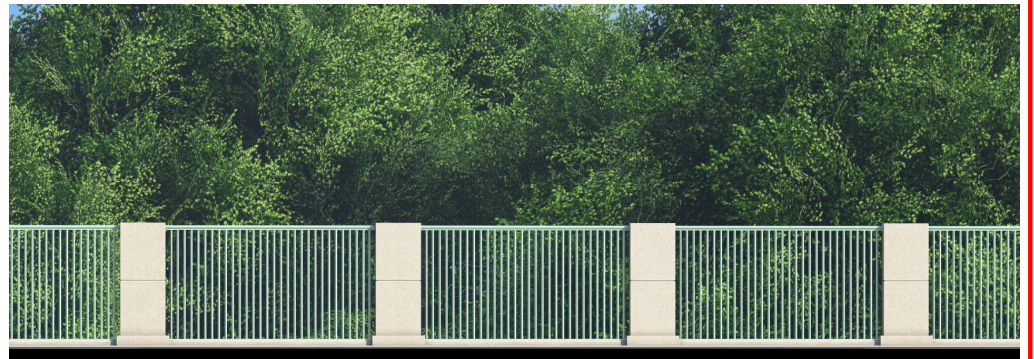
Concrete Post with Metal Handrail - Elevation
