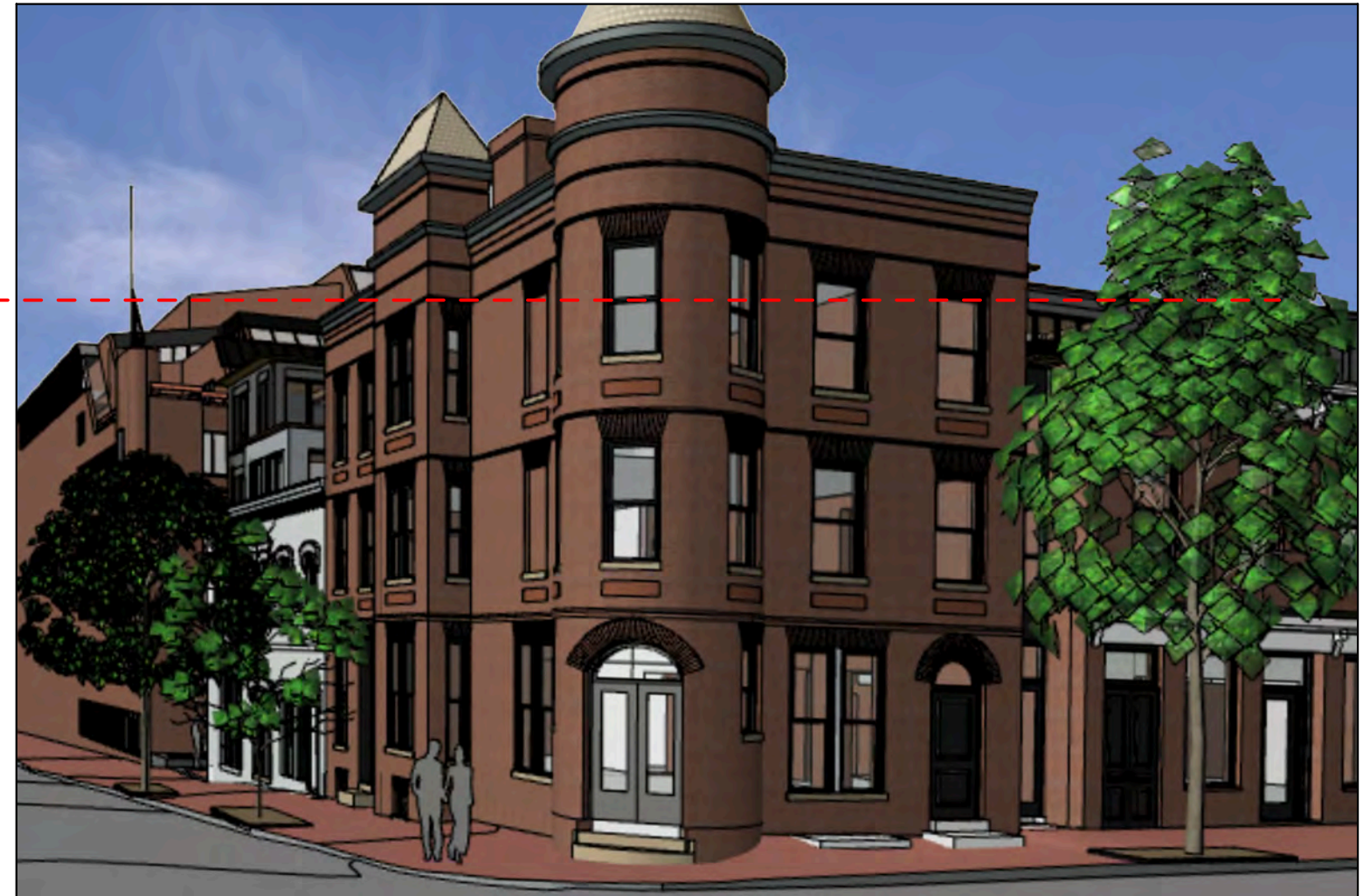
PROPOSED BUILDING BEYOND - BOTTOM OF RED BALLOON IS AT 58'-9", BALLOON IS AT LOCATION OF PENTHOUSE ROOF INDICATED BY DASHED LINE
