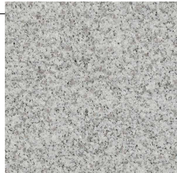
MEMORIAL PLINTH AND STAR BASE WHITE MT. AIRY GRANITE
