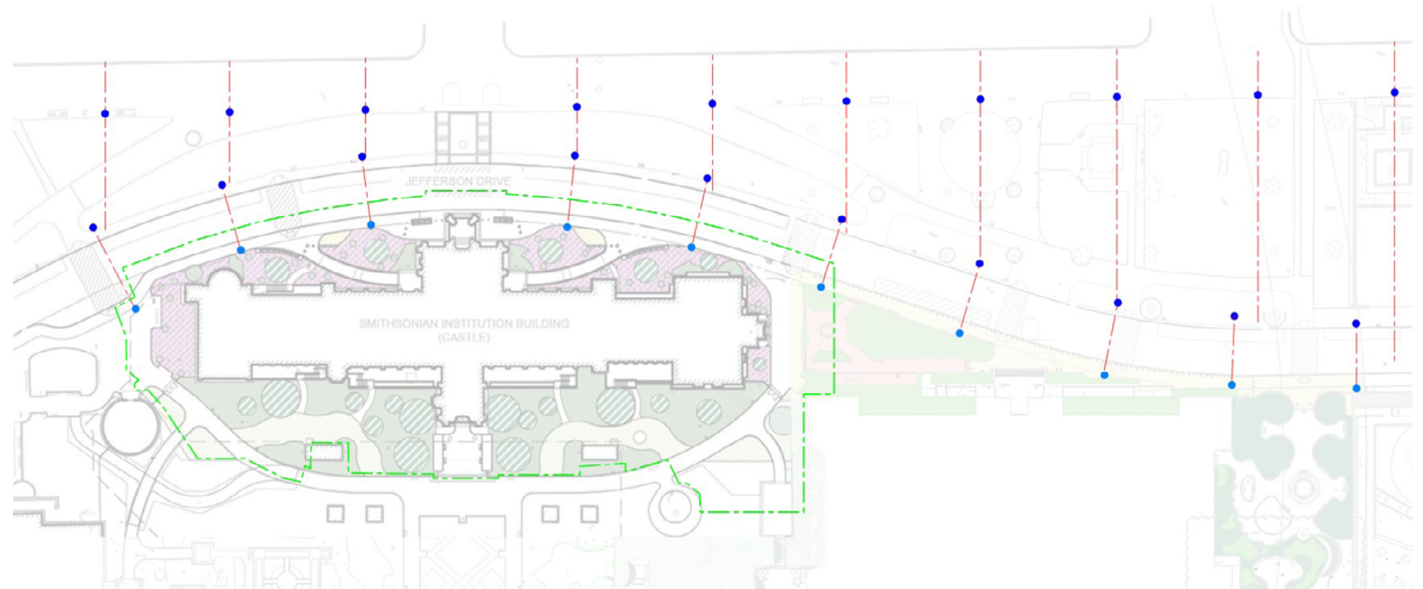
Figure 3.3.4.c – Proposed placement of the Olmsted light posts on the south side of Jefferson Drive, aligning radially with the existing National Mall Olmsted posts
