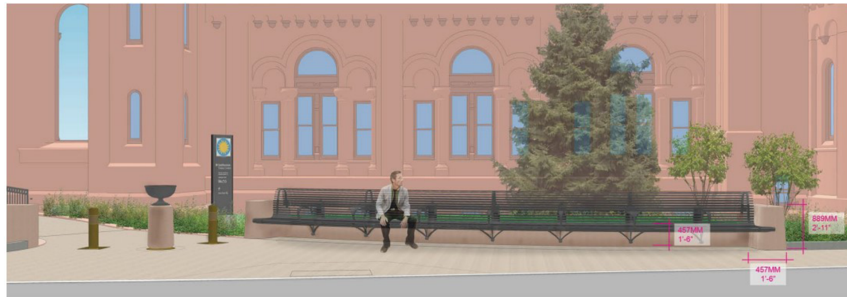
Figure 3.3.2.f – Detail elevation of double-sided metal slat bench at porte cochere
