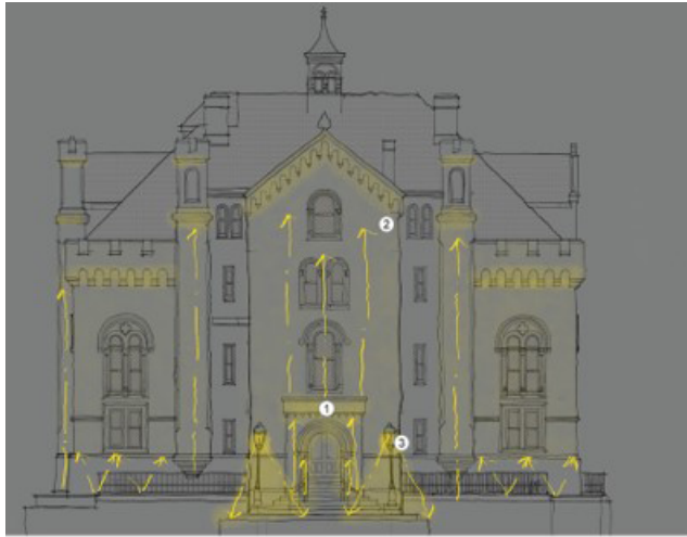
Figure 3.3.4.j - East elevation facade lighting - proposed
