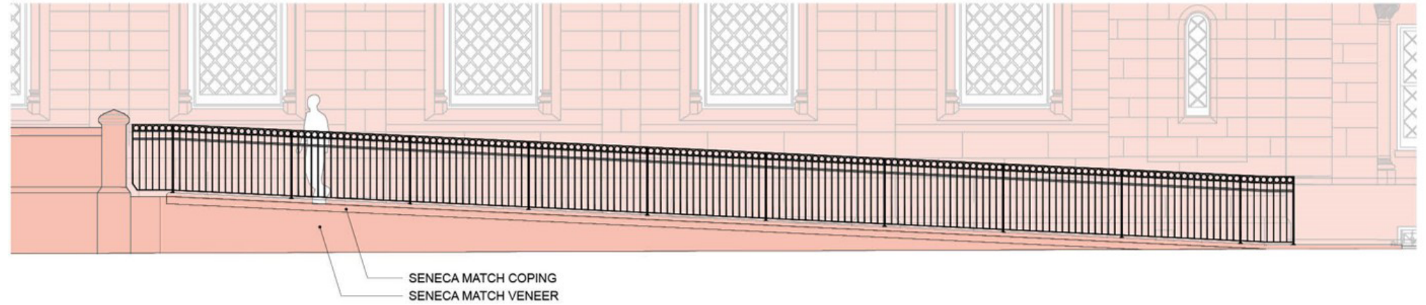
Figure 3.3.6.d – Proposed North Entry accessible walk guardrail elevation
