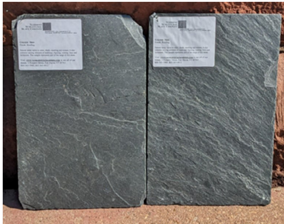
Figure 3.4.2.b – Proposed “Grayson Slate” shingles
