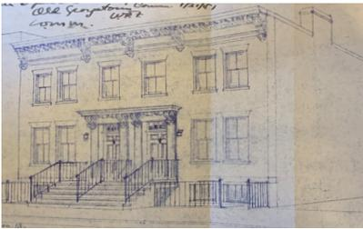
An architectural drawing of the same houses in the photo (right), from 1951 showing the original window style as two-over-two. CFA staff will conduct research to determine the historically correct style of windows for a property.
