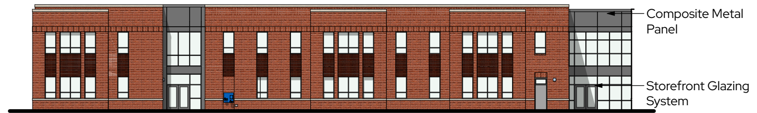
Partial East Elevation
