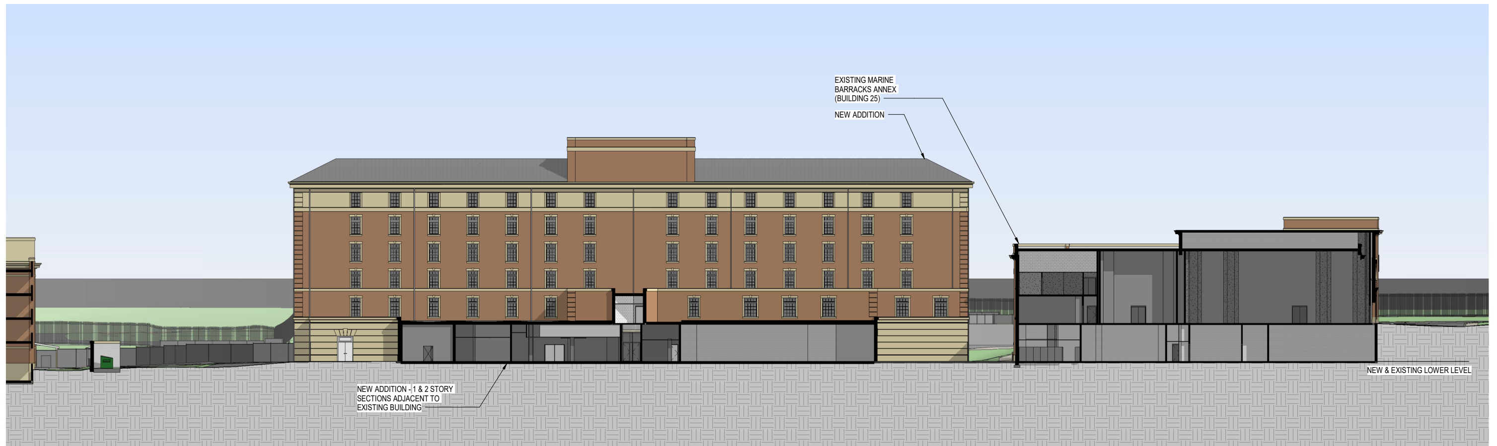
1 SOUTH BUILDING ELEVATION - ADDITION SCALE: 1" = 20'-0"
