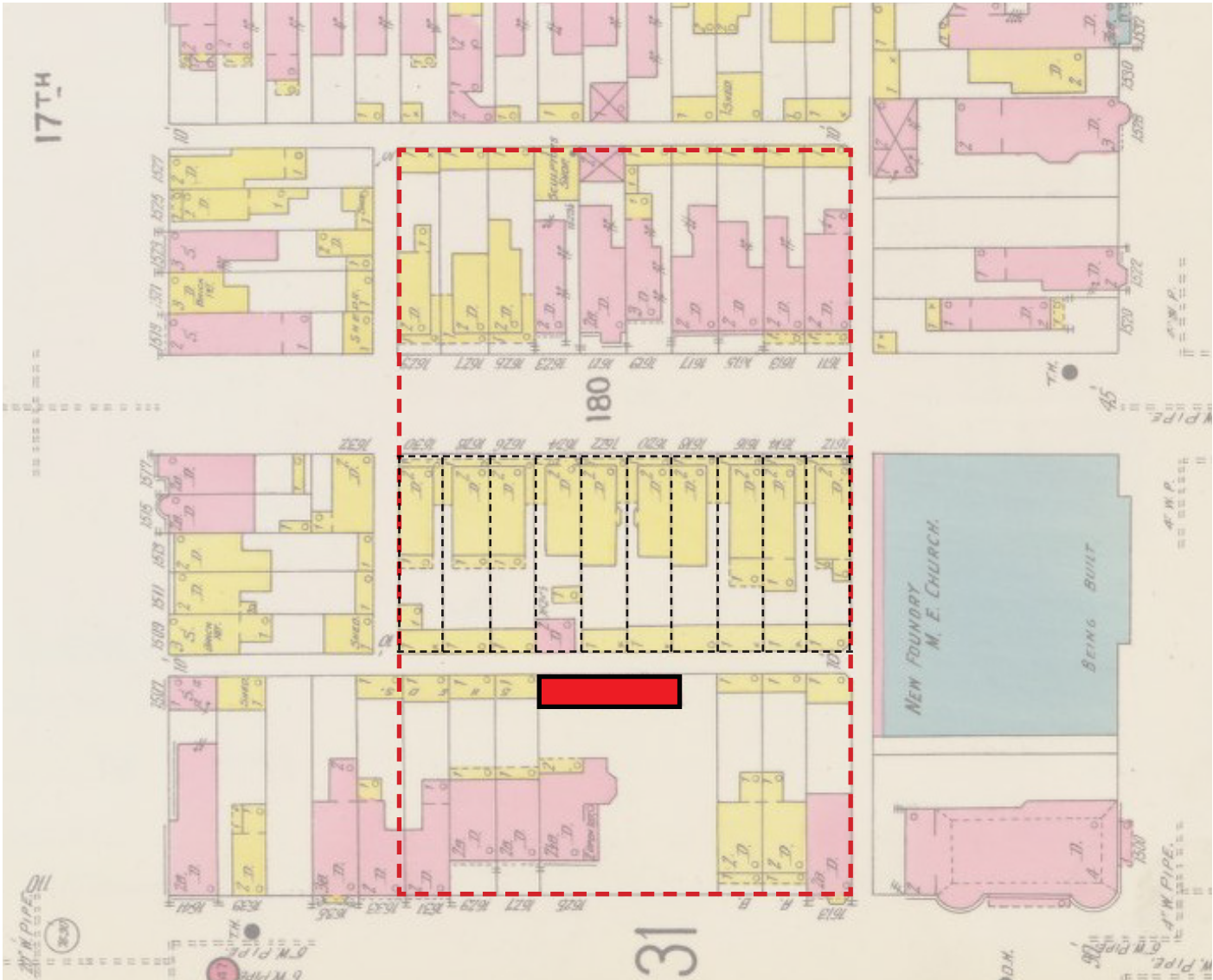
RE-INTRODUCE ORIGINAL HISTORIC LOT LINES AS STRUCTURAL GRID IN FORMER LOCATION OF HISTORIC BUILT FABRIC
