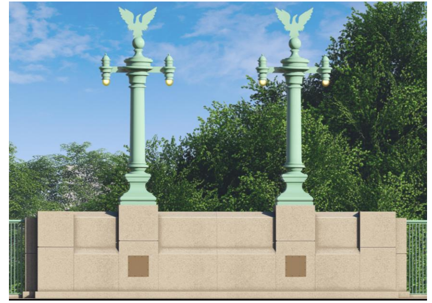
Elevation at Double Light Pole
