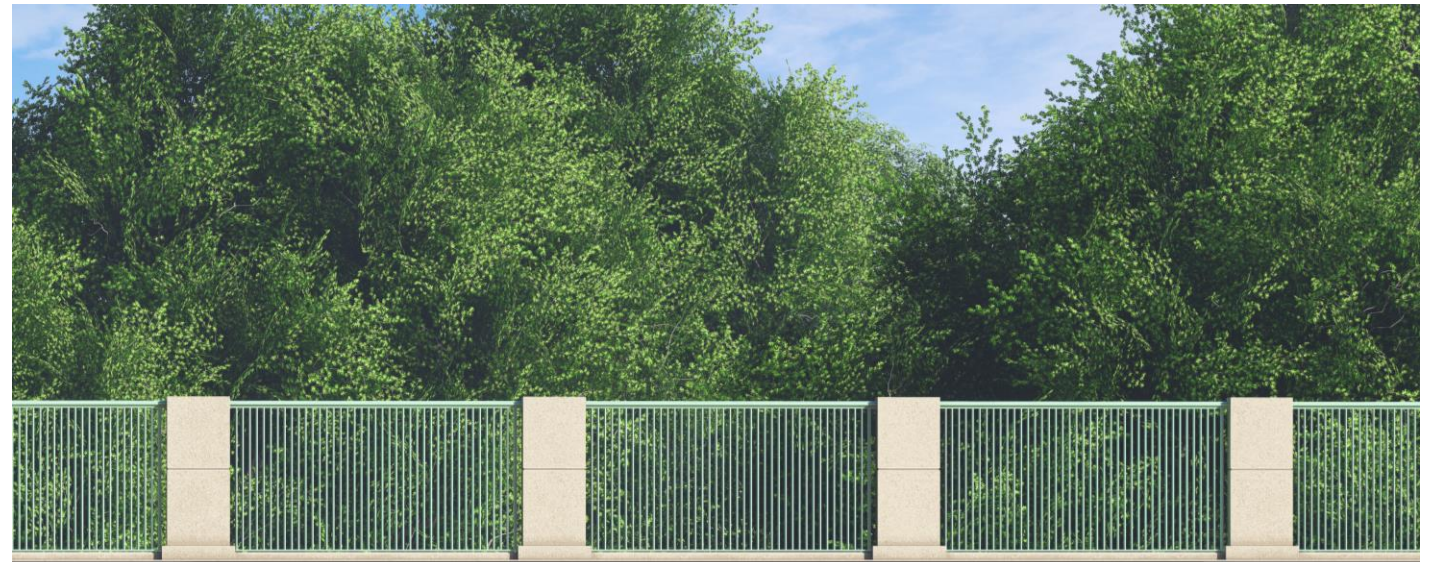
Concrete Post with Metal Handrail - Elevation
