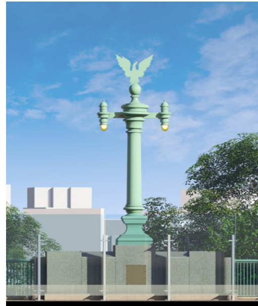
Elevation at Single Light Pole
