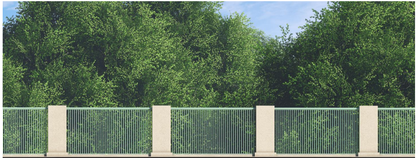
Concrete Post with Metal Handrail - Elevation
