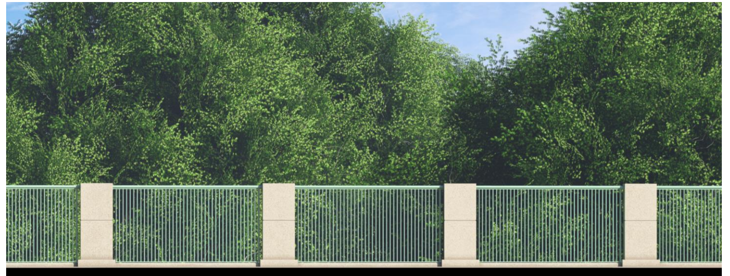
Concrete Post with Metal Handrail - Elevation
