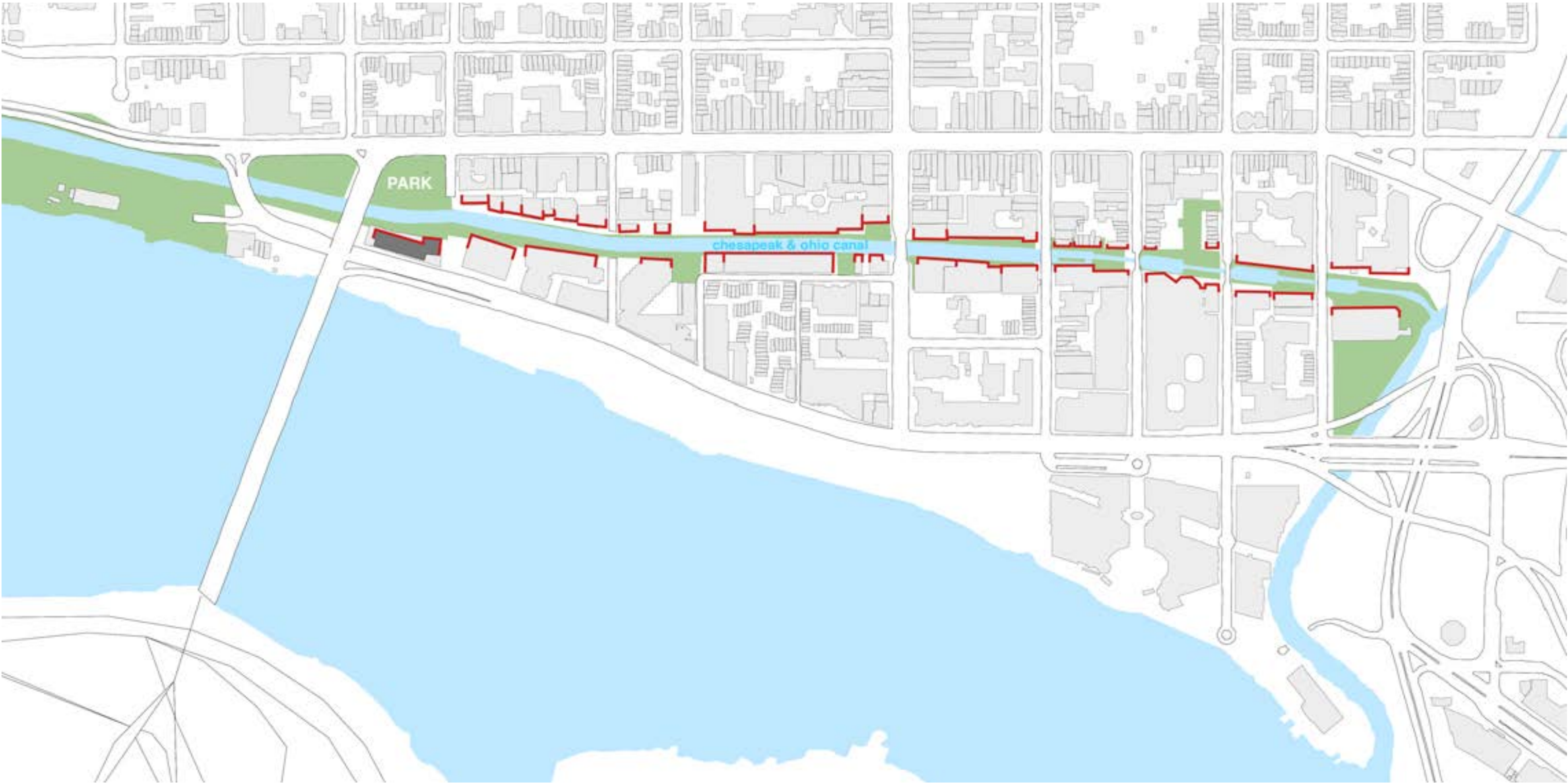
Along the C&O canal the new massing proposal needs to address the small scale of the old industrial buildings of Georgetown. The overall massing of the building therefore shows two sides: the large scale facing the waterfront and a smaller scale facing the Canal.
