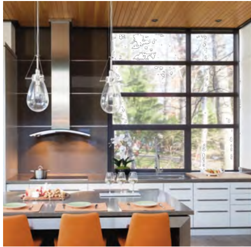
PELLA ARCHITECT SERIES CONTEMPORARY WOOD FIXED + AWNING WINDOW THERMAL LOW-E GLAZING PAINTED TO MATCH EXISTING ADDITION
