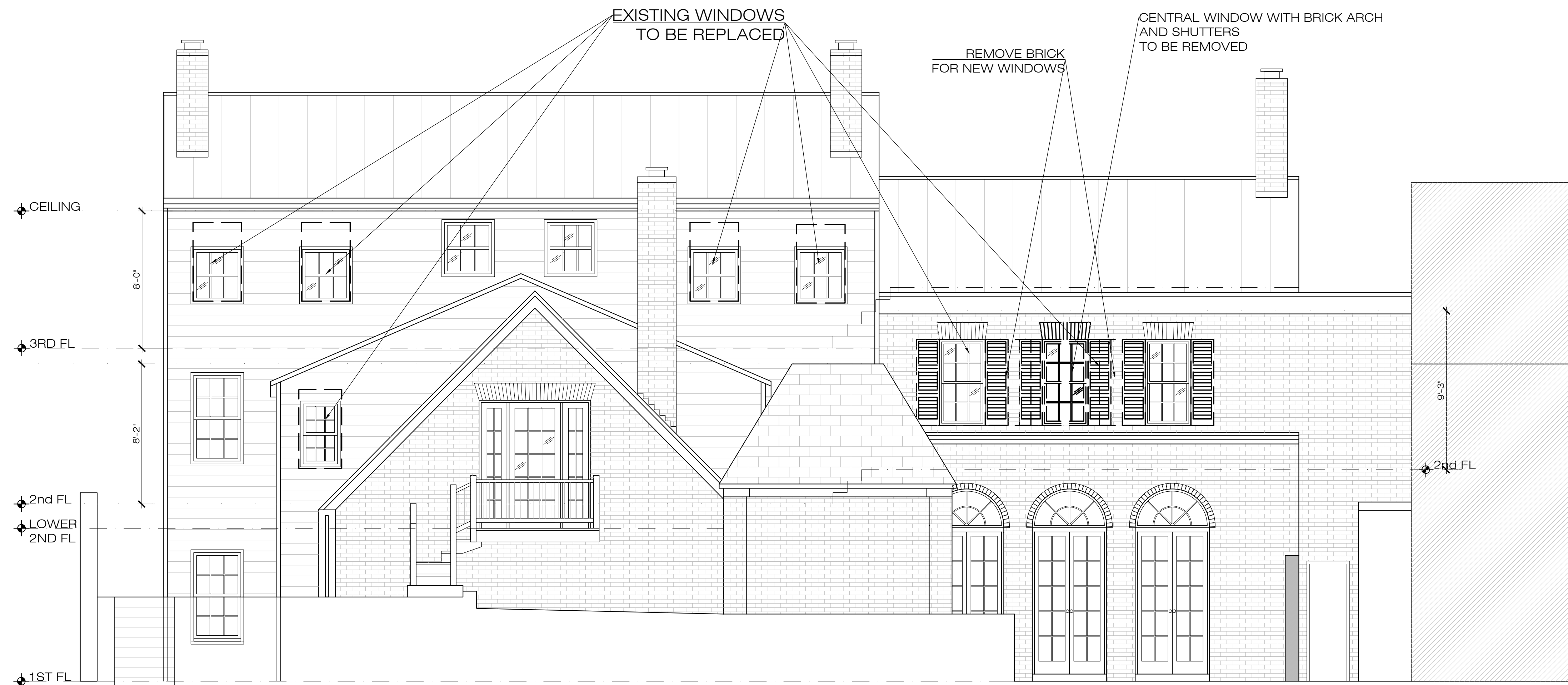
1 MAIN HOUSE EXISTING REAR ELEVATION 1/4" = 1'-0"
