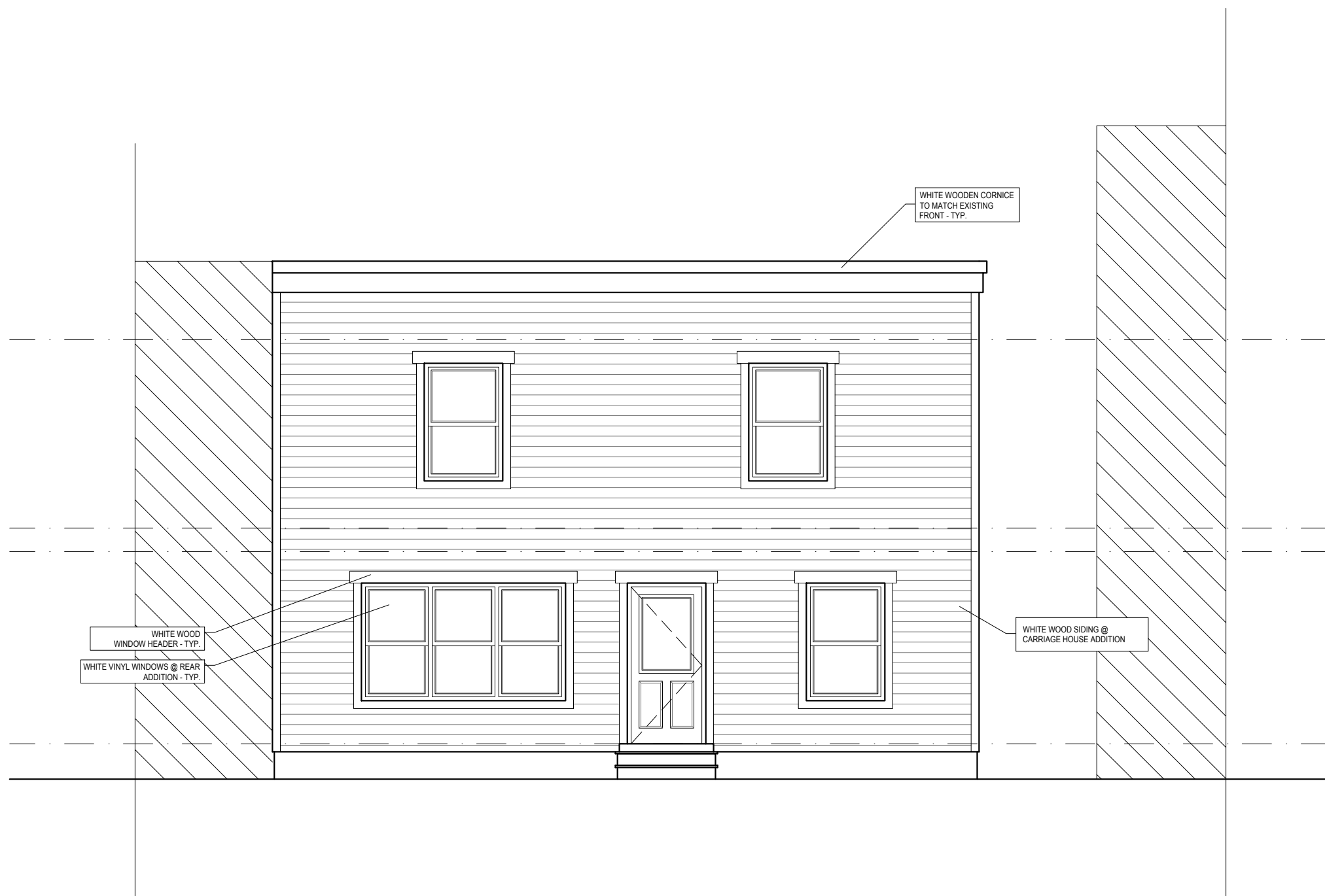
8 CARRIAGE HOUSE PROPOSED REAR ELEVATION SCALE: 3/16" = 1'-0"
