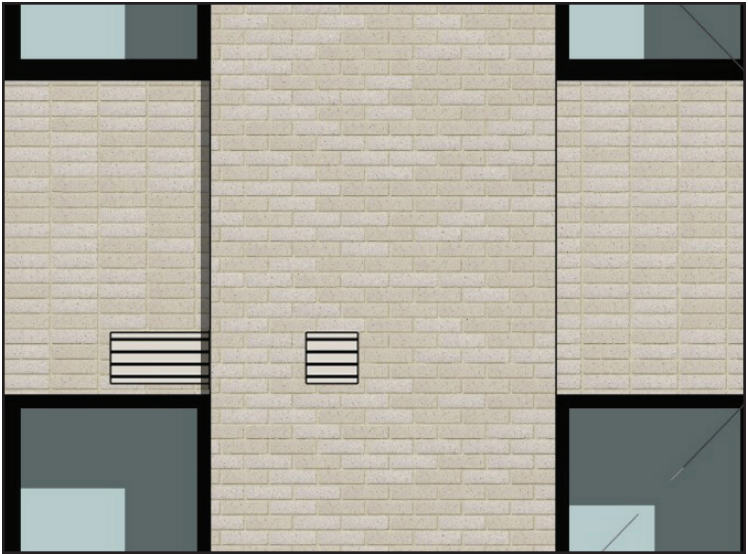
F: Stacked Brick at the Windows on the Brick Facade
