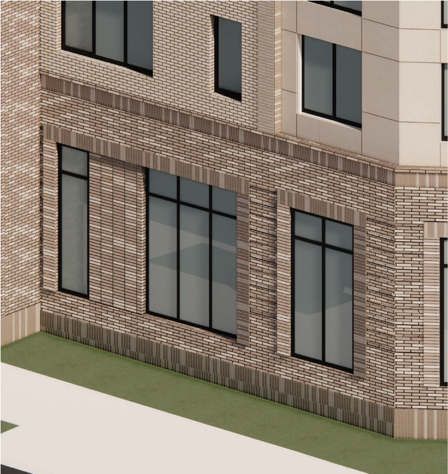
Fenestration details at ground floor openings
